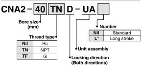
\* The lock unit for a long-stroke cylinder is only applicable for flange type with bore size ø50 to ø100 and storoke 1001 or more. (Example: CNA2-100D-UAL)
