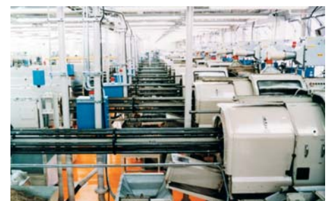
Machining line (6-axis automatic machine tools)
