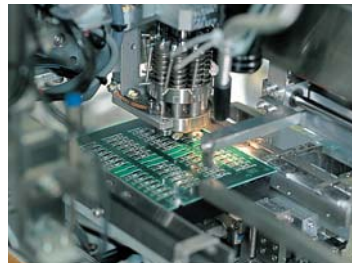
IC chip, being mounted on printed board
