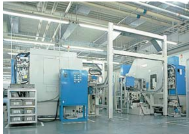
Loader, supplying work for part machining
