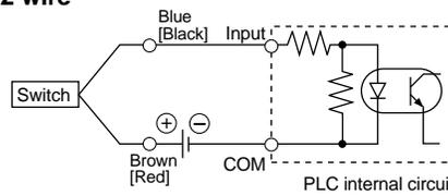
Connect according to the applicable PLC input specifications, as the connection method will vary depending on the PLC input specifications.
