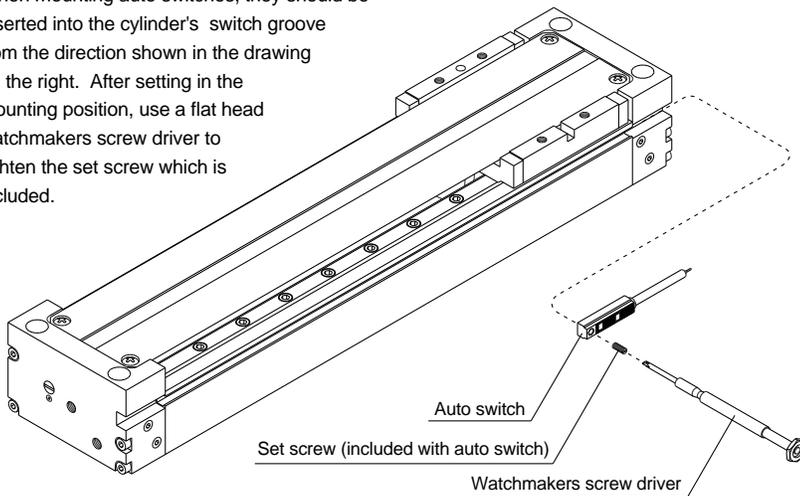
Note) When tightening the auto switch set screw (included with the auto switch), use a watchmakers screw driver with a handle about 5 to 6mm in diameter. The tightening torque should be approximately 0.05 to 0.1N·m. (0.04 to 0.07 ft·lb)
