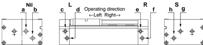
Note) Plugs are installed in ports other than those indicated for the model.
