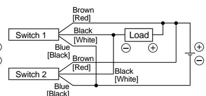
The indicator lights will light up when both switches are turned ON.
