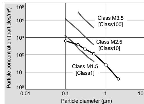
Note 1) This chart indicates the level of cleanliness inside the measurement chamber.
